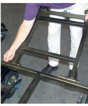
12. All gangs and the push frame should be attached and secure.
