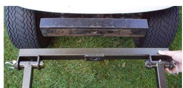
14. Place bolt through the push frame assembly with washer as shown. Tighten nut on the back side until snug, then "back off" nut one quarter turn to allow the Harvester to pivot independently from the vehicle.
