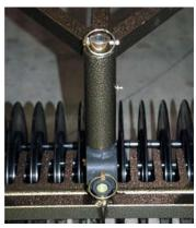
6. Remove the pin collar, and pin from the shaft on the next two gangs behind the front gang.
