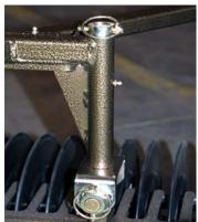
9. Remove pin from the arm assembly and attach the arm to the A-Frame as shown, then re-insert pin. Repeat this process for each arm assembly. (five gang only)
