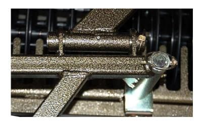
10. Remove pin collar and pin from the rear gang. Slide arm assembly onto shaft, and replace pin collar, and pin to the top of the shaft as shown. Repeat for remaining gang. (five gang only)
