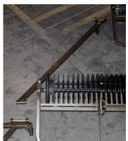
3. On the front gang (with Front Gang Pin) assembly, remove the pin and pin collar from the shaft, leaving the spring as shown in the diagram.
