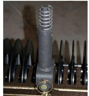
4. Slide the A-Frame over the shaft and spring. You may need to push down on the assembly to get the required space at the top of the shaft to insert the pin collar and pin. Insert pin collar and pin as shown in the diagram.
