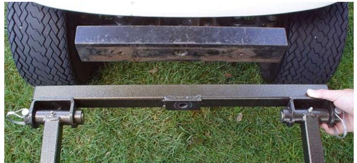
14. Place bolt through the push frame assembly with washer as shown. Tighten nut on the back side until snug, then "back off" nut one quarter turn to allow the Harvester to pivot independently from the vehicle.
