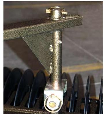
11. Remove the two pins from the rear of the A-Frame. Insert the push frame (as shown) into the space provided. Insert pins and be sure mount is secure.
