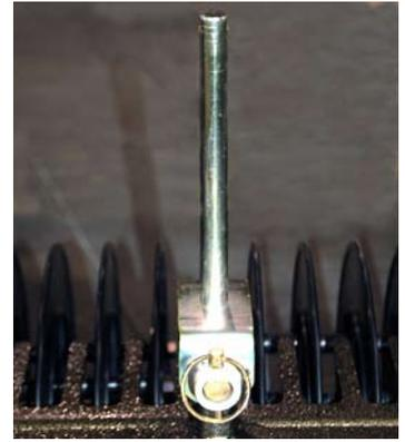
7. Slide A-Frame onto shaft. Then attach the pin collar with the pin as shown. Repeat for each of the two gangs behind the front gang.
