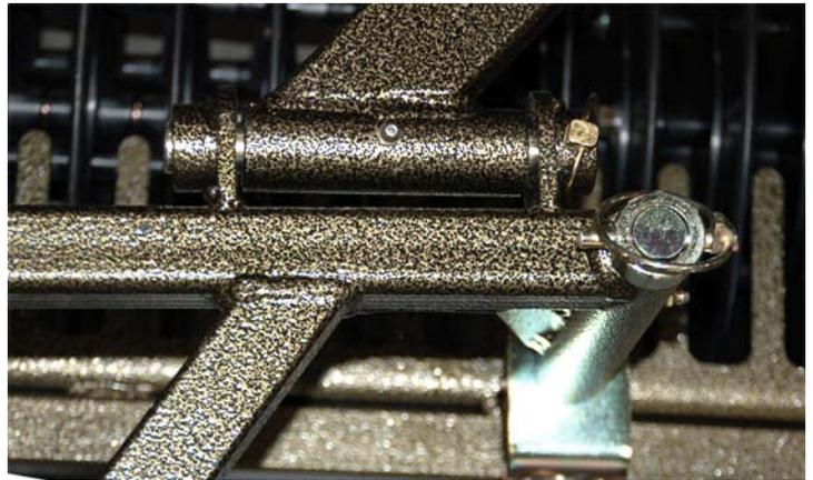
10. Remove pin collar and pin from the rear gang. Slide arm assembly onto shaft, and replace pin collar, and pin to the top of the shaft as shown. Repeat for remaining gang. (five gang only)
