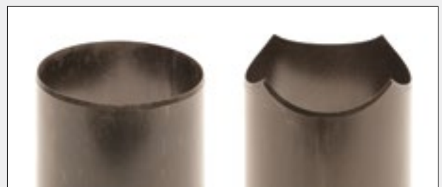
Outside sharpened: push up native soil
